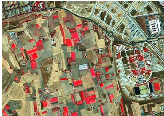
Figure 3: SPOT5 image form the PNT 2005 coverage. Infrared false colour. Pixel size 2,5 m (“Pansharpened”).
