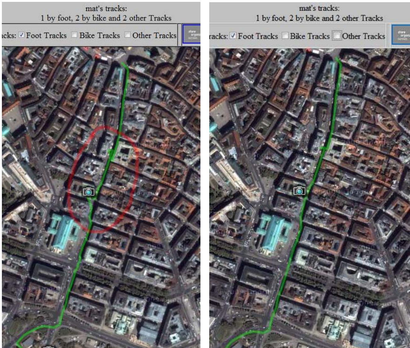
Figure 5: Tracks with smoothing algorithm (right) and without (left).
